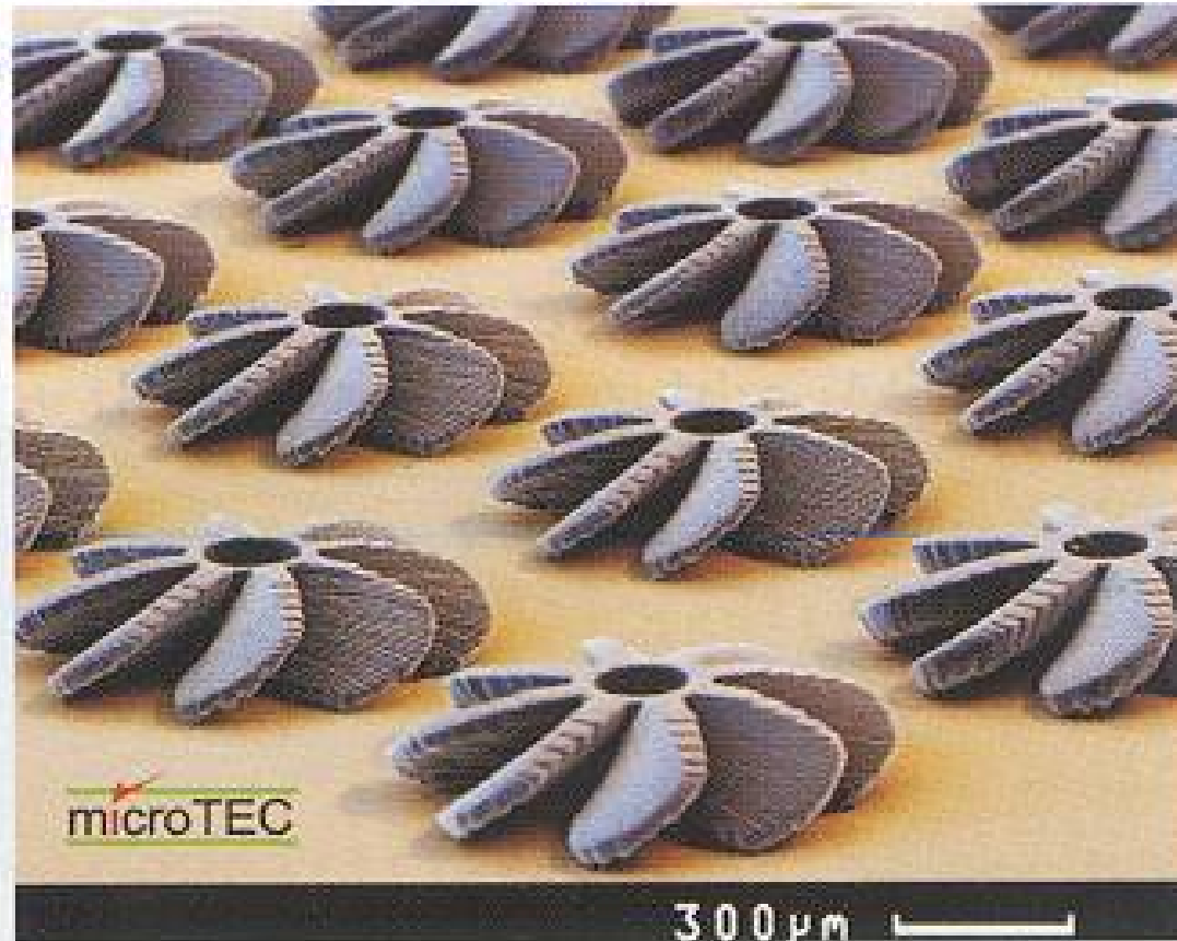
Fig. 1: parallel-produced impellers for flow sensors
